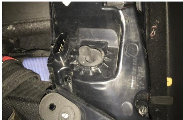
Figure 5: Bulb Holder (Installed)
