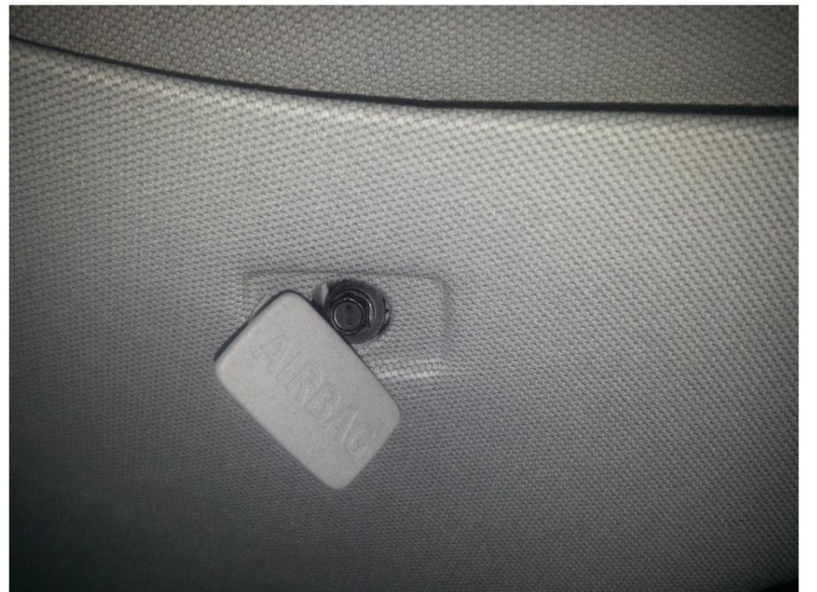
Use a flat bladed tool to release the retainer from the C-pillar panel.
