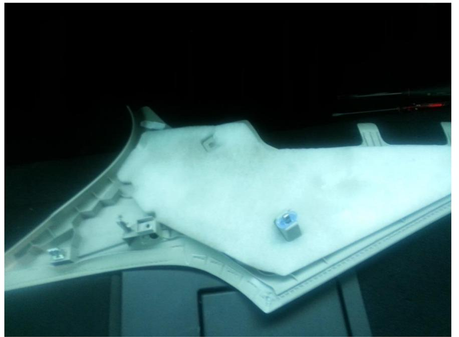
When the screw is off pull the C-pillar panel towards you carefully until the 3 brackets are off, and then pull it in the direction of the front of the car.
