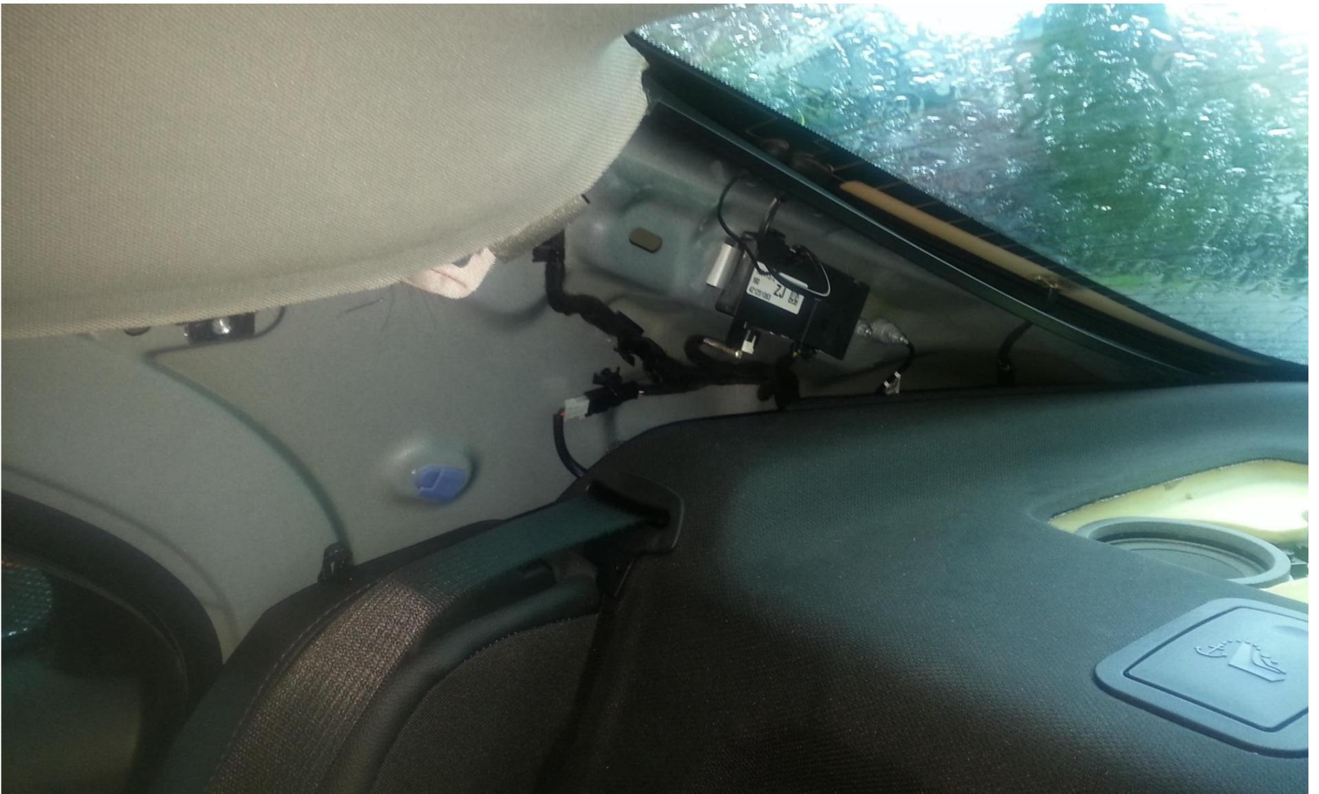
Disconnect the white electrical connector in the middle of the picture above (use a small flat bladed tool to unlock the connector).
